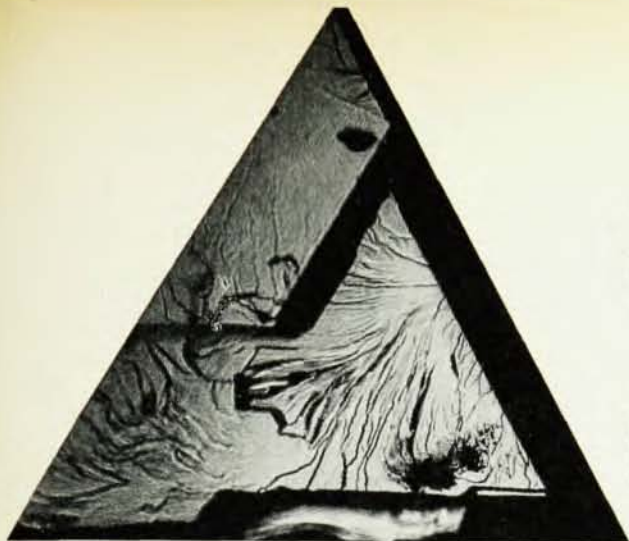
Figure 6. Perfect crystal fragment outlined by crystal planes which first behaved in a ductile manner by twinning, as in Figure 3, and then became brittle and fractured. Specimen is 50-50 bismuth-antimony alloy. Magnified 185 times.
