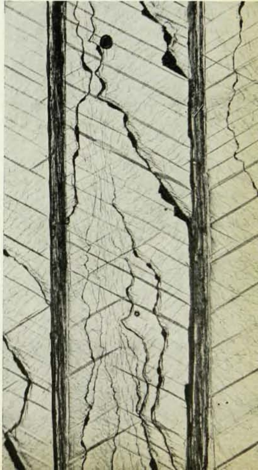
Figure 3. Fractograph of pure cast zinc exhibiting the hexagonal symmetry of the crystal by families of twinning planes intersecting the basal facet. The bands are at exactly 60° to one another. Magnified 80 times.
