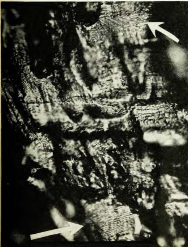
Figure 9. Fractograph of an aluminum alloy (17ST-6) in aircraft construction. A condition of fatigue from many millions of stress reversals has filled the entire body of the grain with fine parallel structures (see arrows) denoting readiness for fracture. These markings are a recent discovery and are not yet solved. Magnified 840 times.
