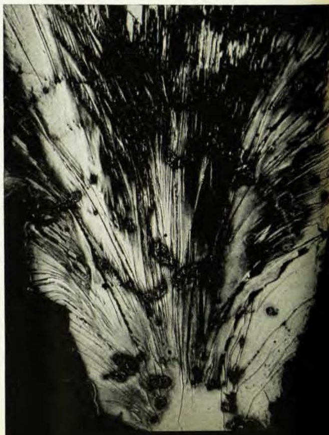
Figure 8. Unsolved fractographic pattern for pure cast antimony fractured at 200°C. The deformation and fracture of this crystal have involved phenomena which are not yet solved. Magnified 65 times.
