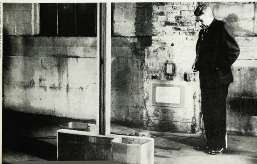
Demonstrating gravitational attraction. In this photo from the PSSC film Forces , Zacharias shows how two boxes of sand deflect bottles of water mounted on a meter stick suspended from an extremely long ribbon of magnetic recording tape. The markings on the wall indicate the undeflected position of a reflected spot of light and its position after the boxes of sand were put in place. The meter stick and bottles can be seen dimly inside the case that shields them from drafts and electrostatic disturbances.
