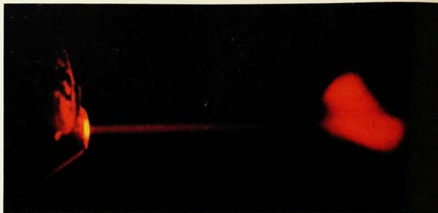
About 500 optically trapped sodium atoms produce the tiny yellow spot barely visible near the top of the fluorescent orange cloud at the stopped end (right) of a beam of neutral sodium atoms at Bell Labs. The cloud is a much larger collection of sodium atoms milling around in the "optical molasses" created by the intersection of six laser beams. The tiny optical trap lurking in the midst of this molasses is formed by the sharp focus of a seventh laser beam, whose optical-dipole gradient force holds the trapped atoms in place for several seconds. The optical molasses has cooled the stopped atomic beam to 300 \mu K. The optical-dipole confining volume is a minuscule 10^{-9} \text{cm}^3 , so that the 500 captured atoms represent an extraordinary density of 5 \times 10^{11} \text{cm}^{-3} . The atomic beam was brought to a halt in the molasses by the radiation pressure of yet another laser beam, shining directly into the oncoming atomic beam. In this vacuum environment, the laser beams are not directly visible.
