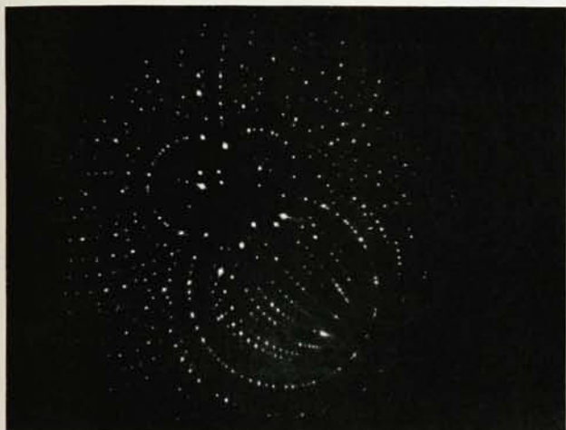
Protein diffraction pattern. Today's powerful x-ray sources and computers permit elucidation of the structure of very large proteins at high resolution from intricate patterns such as this.
