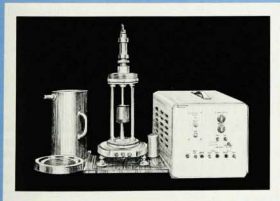
Coal Research—measures volumetric changes as a function of temperature at elevated pressure.
