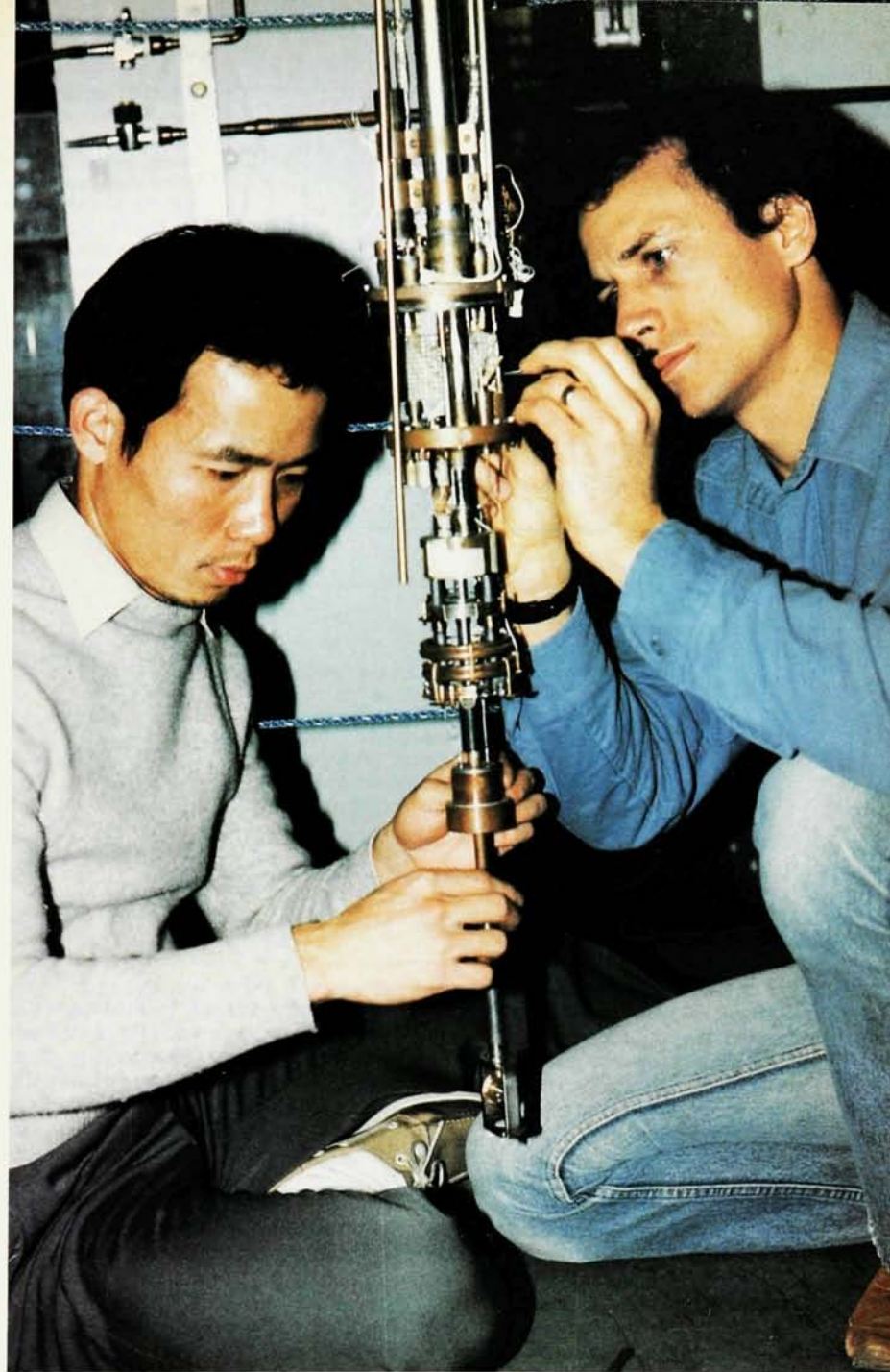
Dilution refrigerator for cooling f -electron materials to millikelvin temperatures. Here graduate student Jenq-Wei Chen and postdoctoral research physicist Steven Lambert prepare the \text{He}^3\text{-He}^4 refrigerator for measurements of the upper critical magnetic fields of heavy-electron superconductors.
