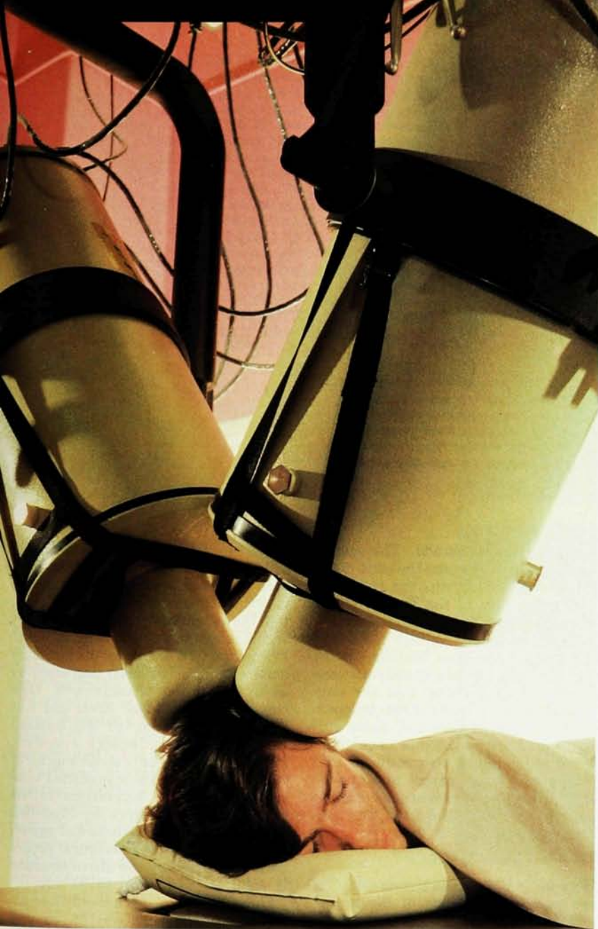
Biomagnetism. SQUIDS inside the two cryostats shown in this photograph detect magnetic fields emanating from the subject's brain. Each cryostat contains seven second-order gradiometers to detect the signal, and three magnetometers and one first-order gradiometer for electronic cancellation of background noise. The sensors are immersed in liquid helium, which is contained by the superinsulated fiberglass cryostats. (Photograph by Hank Morgan, courtesy of New York University Medical Center and Biomagnetic Technologies Inc.) Figure 1
