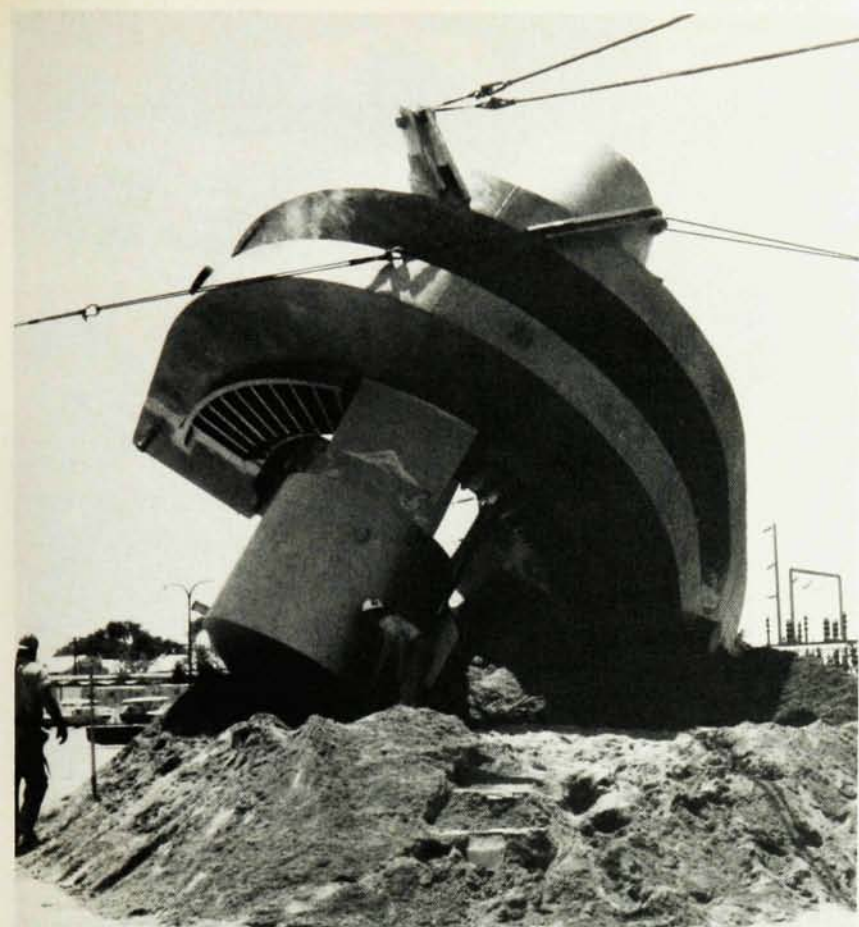
The yin-yang coils that plug the ends of the MFTF-B tandem-mirror facility at Livermore are the largest superconducting magnets in the fusion program. This 340-ton, nested pair of yin-yang coils, seen before installation, provides the complex 8-tesla field that plugs one end of the mirror machine. A second pair plugs the other end. The entire magnet system of the MFTF-B was successfully tested last month, just in time for the project to be relegated to standby status by budget cuts. Figure 6
