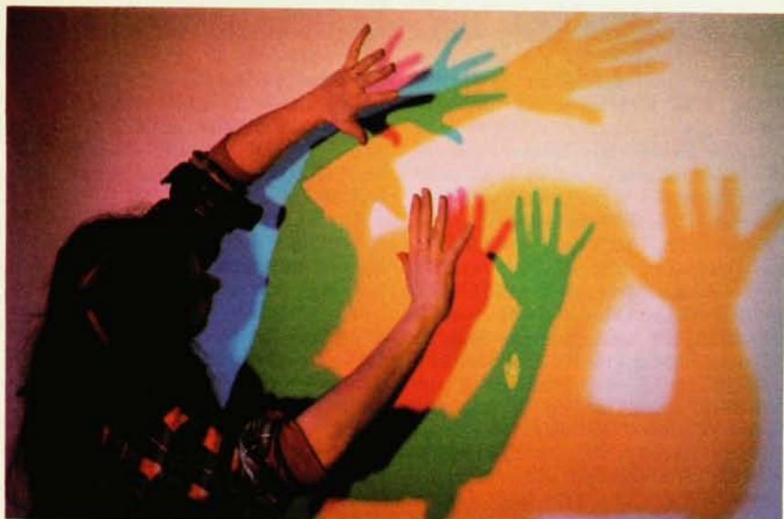
In this Exploratorium exhibit, spotlights cast primary red, blue and green light against a wall, where they combine to make white. If one blocks one of the beams, a shadow appears in the white field in the color complementary to the one blocked.
