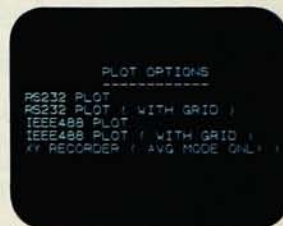
The NIC-370 sends displayed information to plotters for hard copy records.
