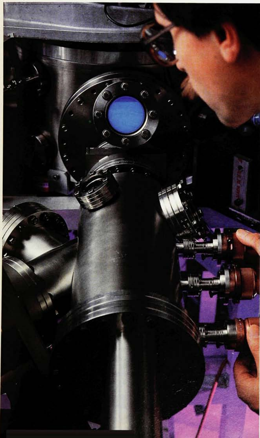
Etching of silicon wafers by an rf plasma (blue glow). In this photo the author is monitoring the process. The vacuum chamber in the foreground contains apparatus for mechanically transferring completed wafers into an ultra-high-vacuum system for further processing and analysis. Figure 1
