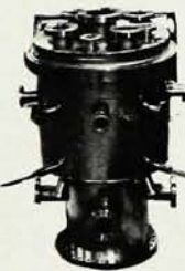
Custom Designed UHV Bell Jar with LN 2 Cooled Furnaces.
