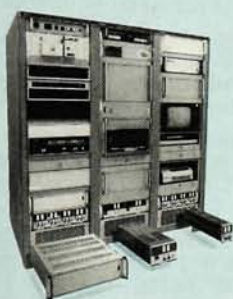
Grumman CAT™ Test System incorporating one SNR 488-8 controlling 11 ATEs.
