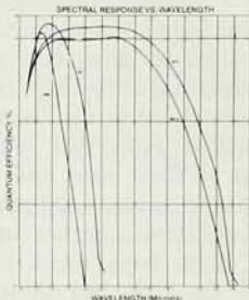
The spectral response of Thorn EMI UV PMTs falls into three groups:
