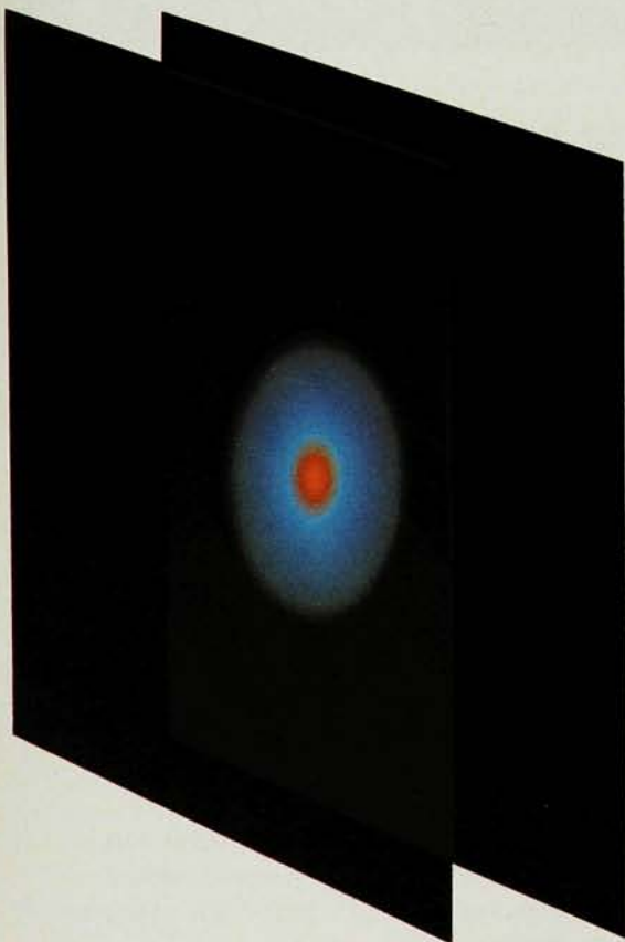
Quantum confined Stark effect , in artist's conception. The drawing on the left shows an electron-hole pair, or exciton, trapped in a quantum well in a superlattice material. The left and right planes represent the walls of the well. When an electric field is imposed, right, the electron (blue cloud) and hole (orange cloud) move apart, but the walls of the well are close enough together to prevent the exciton from ionizing.
