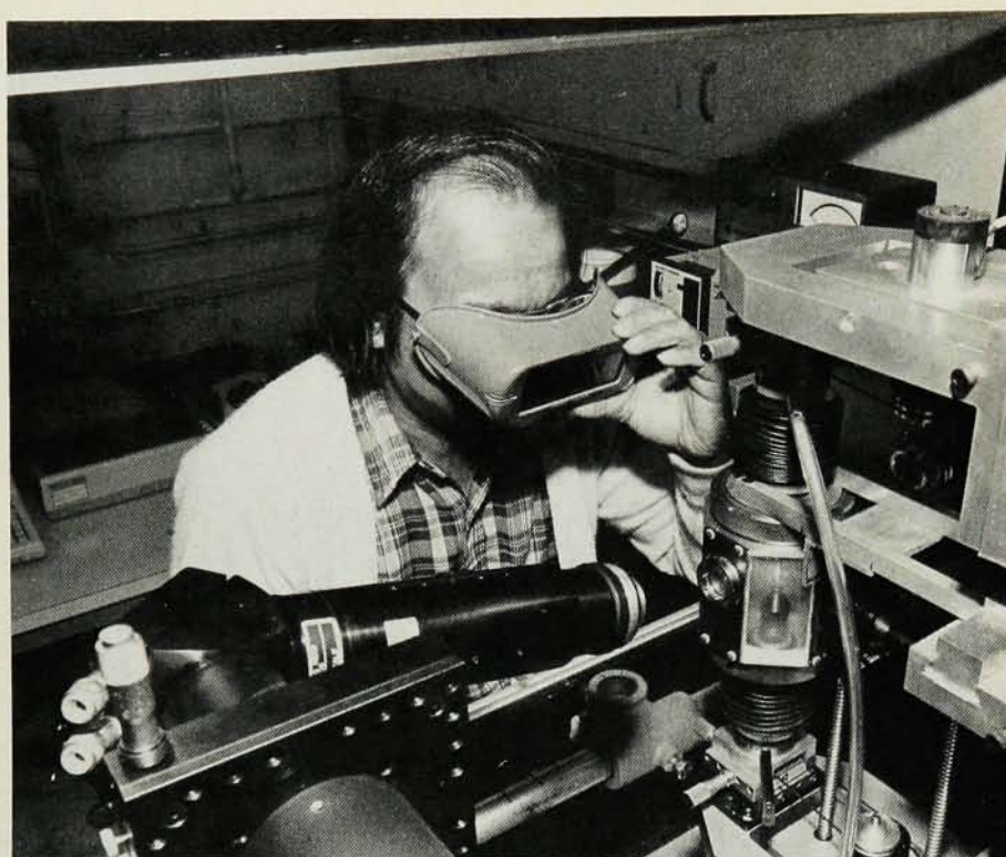
Single-crystal fibers. By continuously drawing material from a "button" heated by a sharply focused CO 2 laser (insert), single-crystal fibers can be created from sapphire and many other compounds. These crystals, which are among the most perfect ever produced, make it possible to study fundamental processes such as eutectic solidification and the growth of metastable phases. The high growth rate and ease of operation make possible rapid surveys of new materials and can provide novel types of fibers for optical devices. The apparatus shown here is in the laboratory of Robert S. Seigelson at the Center for Materials Research at Stanford University. (Courtesy of Roger K. Route.)
