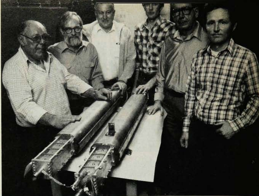
First two superferric magnets developed at the Texas Accelerator Center are displayed here by (left to right): R. Stegman, R. Wolgast, R. Huson, J. Zeigler, H. Hinterberger and J. Colvin. In the SSC, these magnets, each 140 meters long, would be mounted one above the other, carrying the colliding beams in opposite directions.
