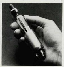
and 1.0 inch (25 mm) in diameter. It produces 0.5 mW of output power at 632.8 nm; the output power stability is  $\pm$  20 %. The output beam is polarized and 0.47 mm in diameter. The polarization ratio is 500:1 and the beam divergence is 1.7 mrad. The operating voltage is 800 to 1000 V dc at 4.0 mA, making battery operation possible. Melles Griot, 1770 Kettering Street, Irvine, California 92714
