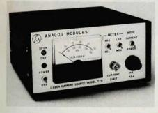
with a front-panel trimmer and select between a constant-current and constant-light-power mode. The large analog meter on the front panel is suitable for absolute and relative measurements. The current (up to 10 KHz) can be modulated through a modulation port. The unit operates on either 120 or 240 V and is priced at \$770. Analog Modules, 125 Baywood Avenue, Florida 32750
