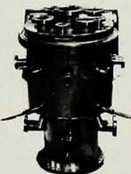
Custom Designed UHV Bell Jar with LN 2 Cooled Furnaces.
