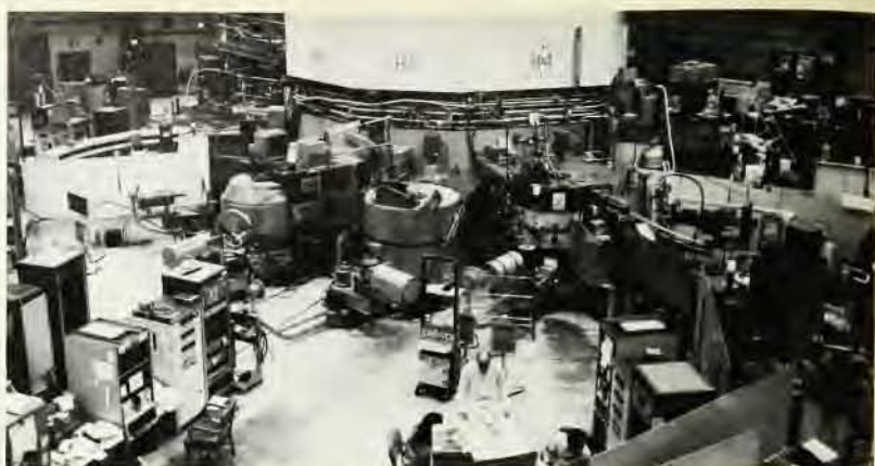
The 60-MW High Flux Beam Reactor at Brookhaven is the only cold neutron source in the US. The new National Research Council report calls for its upgrading.
