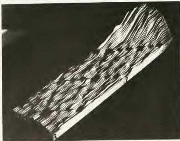
Scanning tunneling microscope data, plotted in three dimensions, and model of surface. The STM plot (left) is of the 7×7 reconstructed (111) surface of silicon at 300 °C. The adatom model at the right has a periodicity consistent with the plot. The plot and model are the work of Gerd Binnig, Heinrich Rohrer, Christoph Gerber and Edmund Weibel of IBM, Zurich. Figure 4
