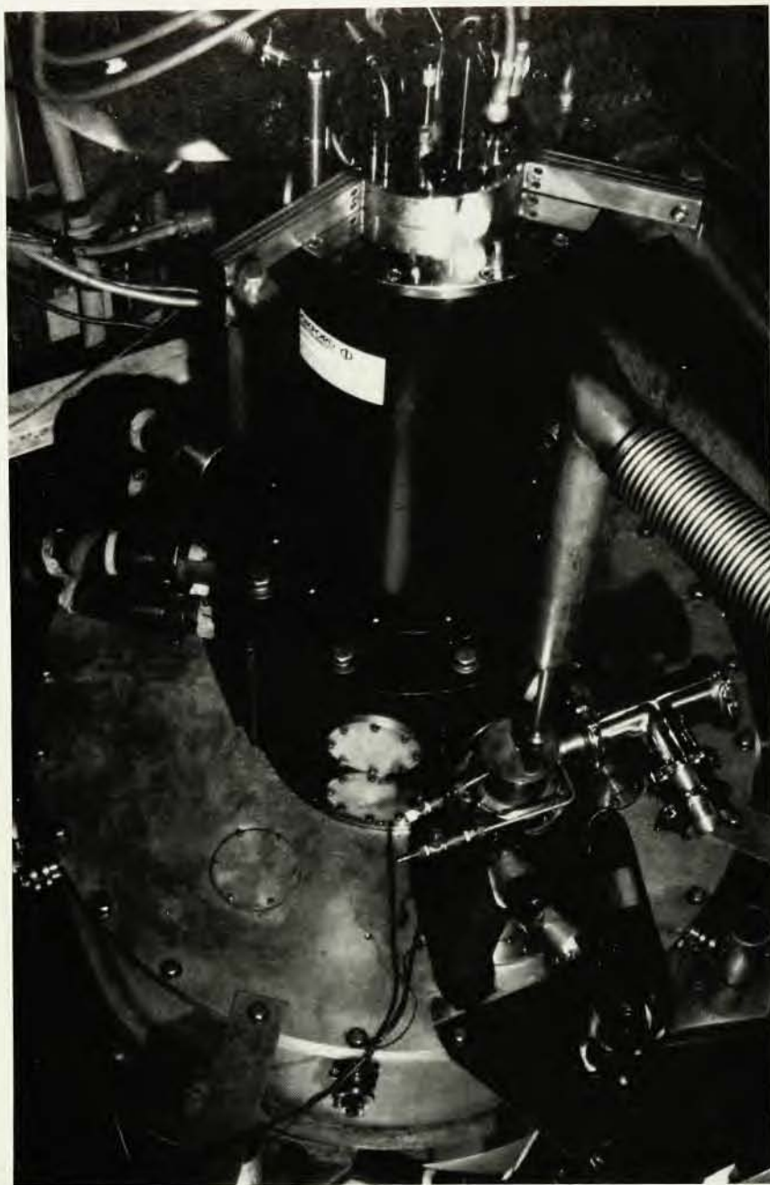
He 3 -He 4 dilution refrigerator sitting in the 3-cm bore Bitter insert of the hybrid magnet. This apparatus produced 85 mK in a 28.5 T field. Figure 4
