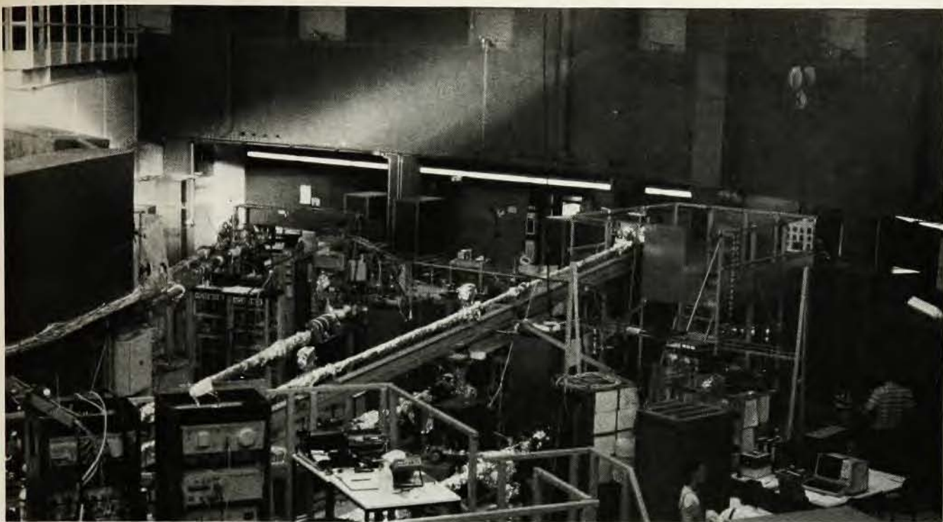
Synchrotron-radiation beam lines fanning out from the storage ring BESSY in West Berlin.
