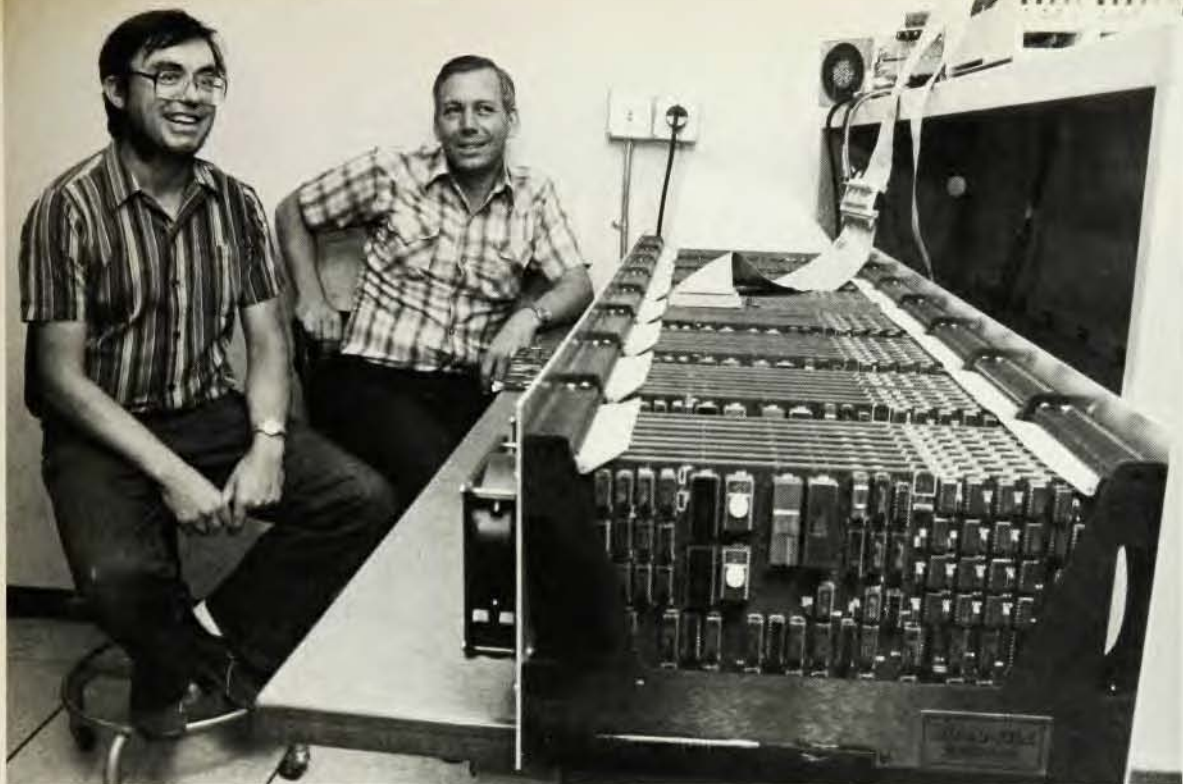
"Cosmic cube." This concurrent processor consists of 64 identical small computers connected so that each can send messages to 6 others. The 64 corners of a 6-dimensional cube, or hypercube, have this connection topology. Each small computer contains 16-bit Intel 8086 and 8087 processors with 136 kilobytes of memory—roughly the power of an IBM personal computer. The $80 000 cube has up to one-tenth the power of a Cray-1 computer, but one-hundredth the cost. Shown here with the experimental machine at Caltech are Geoffrey Fox (left) and Charles Seitz. Figure 2
