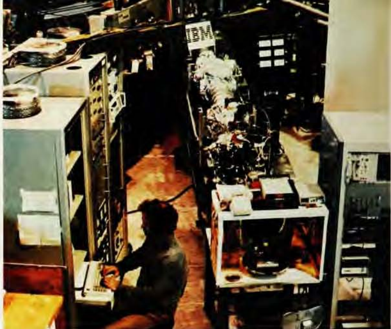
Beam line for x-ray lithography installed by IBM on Port U6 at the National Synchrotron Light Source at Brookhaven National Laboratory. Figure 2
