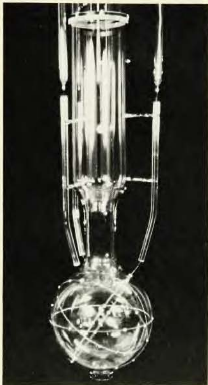
The larger Stanford monopole detector, after a year of operation, has seen nothing like the one apparent monopole signal recorded by its smaller predecessor. Three orthogonal superconducting loops (plus a horizontal calibrating loop), each linked to a squid magnetometer, are wound on a 10-cm-diameter pyrex sphere.
