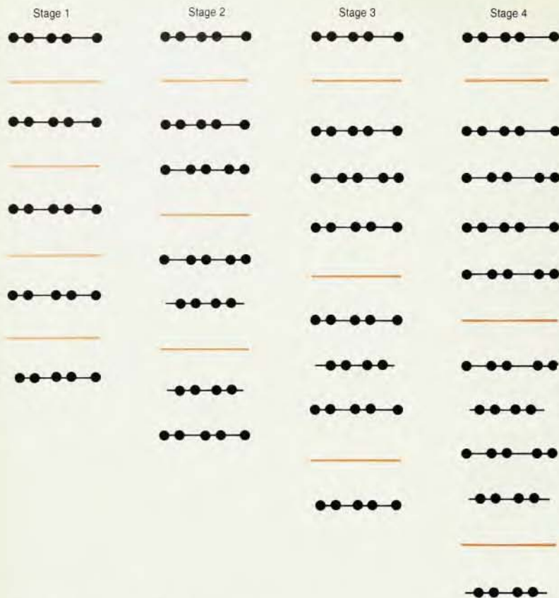
Staging phenomenon. This schematic diagram shows the arrangement of layers in four potassium-intercalated graphite compounds. Solid lines connecting circles represent graphite layers, with the positions of the circles indicating schematically the projected positions of the carbon atoms. The colored lines represent potassium layers. In the stage-one compound, layers of graphite and potassium alternate. In stage- n compounds, there are n graphite layers between successive potassium layers. Graphite layers between potassium layers maintain an alternating pattern of registration, as indicated. The distances I_c between adjacent potassium layers in the stage-one through stage-four compounds represented here are 5.35 Å, 8.75 Å, 12.10 Å and 15.44 Å, respectively. Potassium layers in the stage-one compound arrange themselves in a sequence of four orientations.
