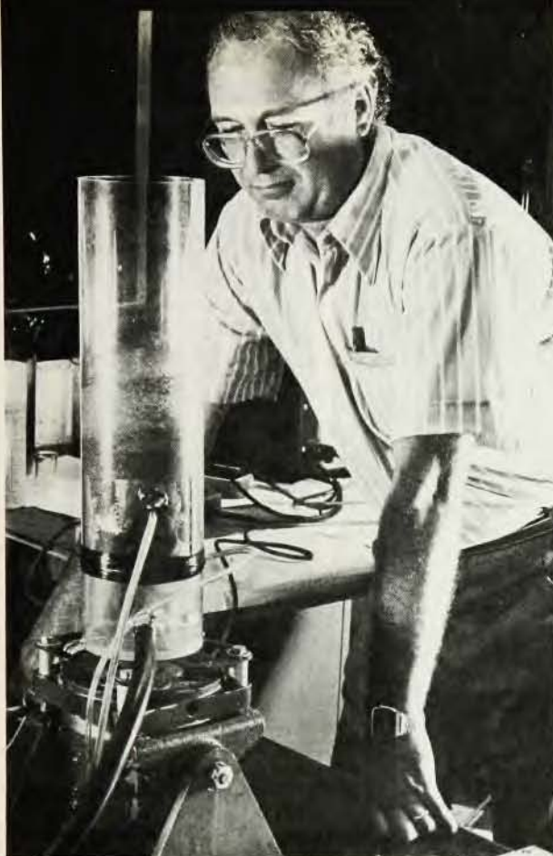
Test of vented compression molding technique , developed under the sponsorship of Martin Marietta Corp. This technique permits ablative materials used on the exterior fuel tank of the Space Shuttle to be molded more reliably and easily than was previously possible. Work began at MIT-Industry Polymer Processing Program.
