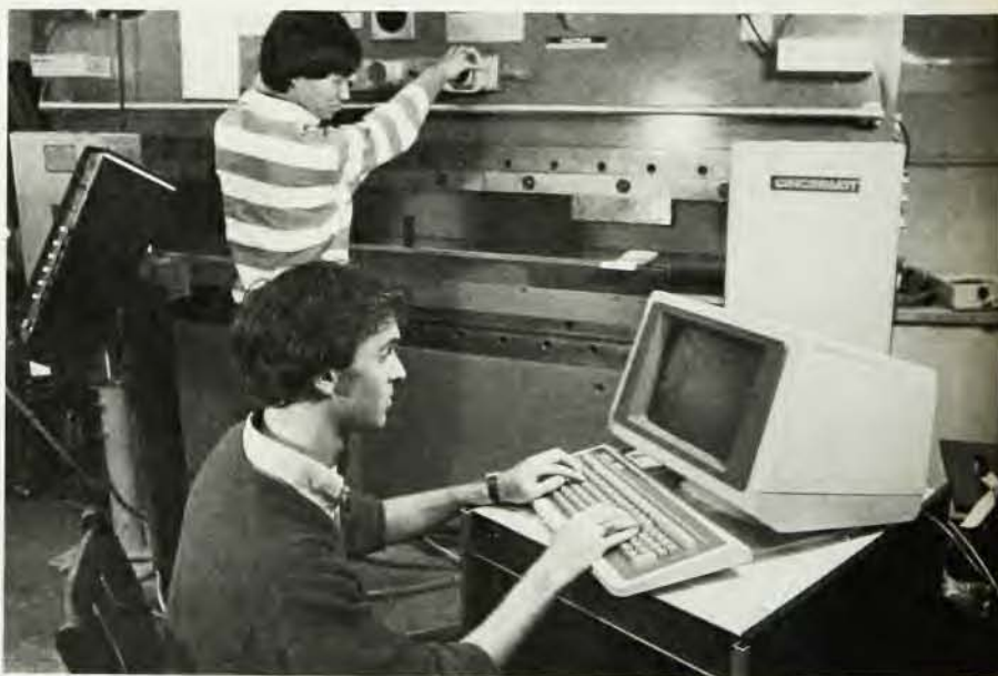
Machine for bending sheet metal —called a brake—is operated by students Bernard S. Chen (striped shirt) and Michael L. Agronin (foreground) at MIT's Laboratory for Manufacturing and Productivity.
