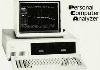
The IBM-PCA provides the ultimate solution to your multichannel pulse height analyzer requirements. By building the hardware on a card which fits inside the computer, we've eliminated the need for an external buffer and expensive NIM system.
