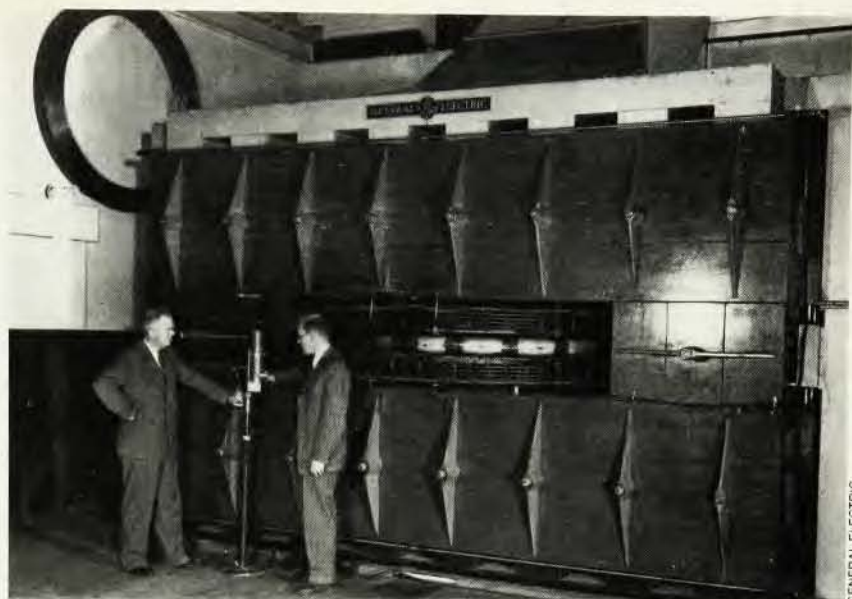
Betatron. Ernest Charlton (left) and Willem Westendorp in 1950 with the 100-MeV betatron they helped design in the early 1940s.
