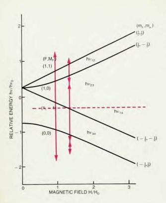
Breit–Rabi diagram for the eigenenergies of muonium in an applied field in a vacuum. At low fields, total-angular-momentum quantum numbers F and  $M_F$  describe the system. At high fields, the muon and electron spins are decoupled and the individual quantum numbers  $m_s$  and  $m_n$  describe the system. The applied field is given in units of  $H_0$ , which is 1585 gauss. The frequency  $v_0$  is 4463 MHz.
