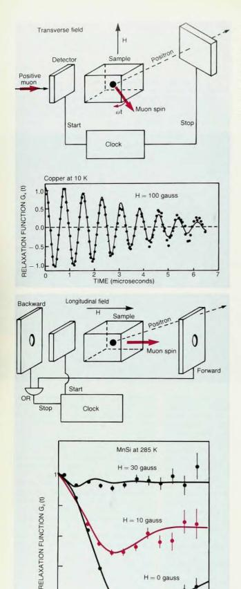
Spin detection schemes and corresponding results. In the setup illustrated at the left, the applied magnetic field is perpendicular to the spins (colored arrow) of the incident muons. In the configuration below, the two are parallel. In either case, the incident muon triggers a detector near the target sample and the decay positron triggers another counter, giving rise to time histograms such as those shown below the diagrams. (Copper data from TRIUMF; MnSi data from reference 7.) Figure 2
