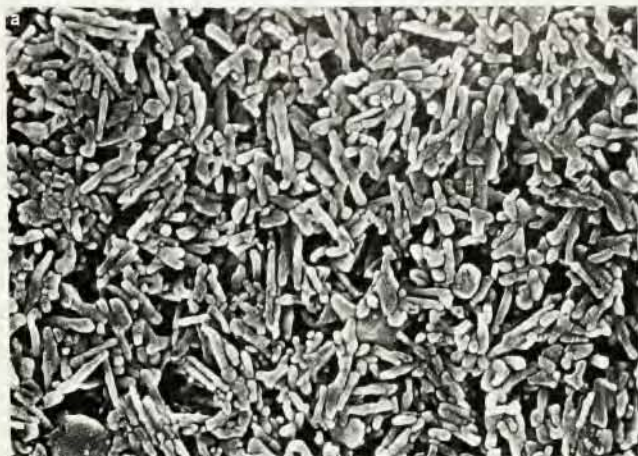
Magnetic tape particles. The electron micrograph in a shows acicular, or needle-like, particles of \gamma\text{-Fe}_2\text{O}_3 in a floppy disk. The micrograph in b shows isotropic magnetic particles in a tape. (Images courtesy of James U. Lemke, Eastman Technology.) Figure 2
