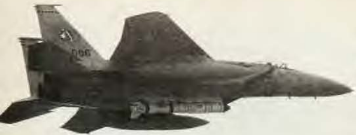
A US Air Force F-15 fighter carrying an anti-satellite missile under its belly. The missile is designed to carry a miniature homing interceptor vehicle into space.
