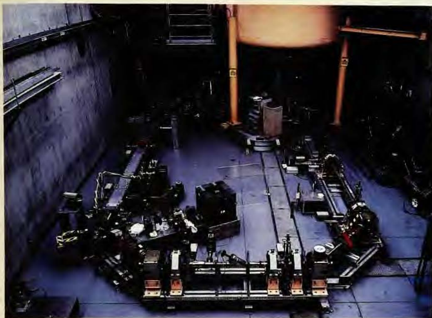
The Santa Barbara FEL produced its first laser output at 400 microns at the end of August. One sees the base of the tall, yellow electrostatic accelerator tank at the back, filled with 6 atmospheres of \text{SF}_6 gas. The beam loop on the floor passes the electron beam through the FEL (left) and recirculates it back to the accelerator (see drawing opposite).
