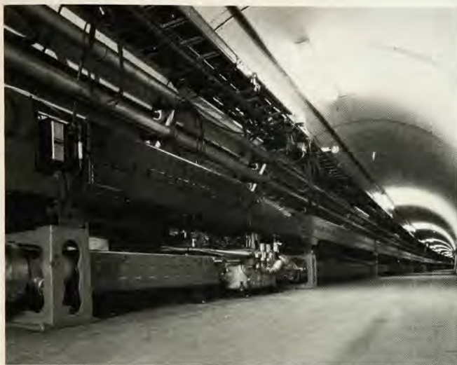
The tunnel of the main accelerator at Fermilab. The newly installed ring of superconducting magnets runs along the floor of the tunnel. These magnets will guide a beam of protons up to an energy of 1000 GeV. Directly above the superconducting ring is the older ring of conventional magnets. Various power and electronics cables run overhead.
