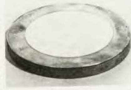
Copper specimen modified by ion implantation in the central region exhibits different surface oxidation rates in the two regions. 4 Other properties of metals and alloys are controlled by implantation, such as bearing wear. The ion-implantation programs are based on the main facilities of INFN in Legnaro (Padova) and the GNSM groups in Trento and Catania. Figure 6
