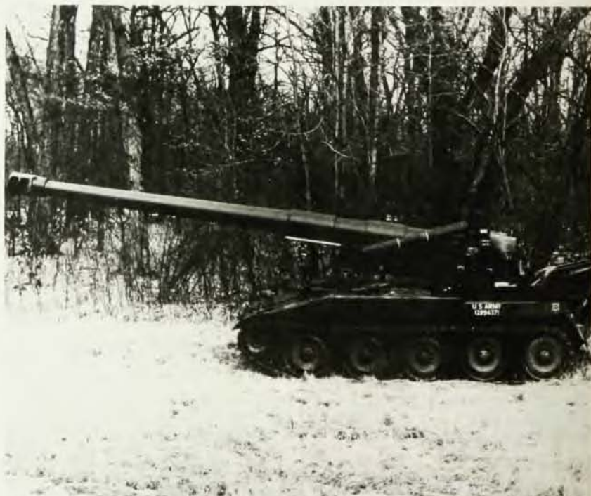
Cannon. This Army photograph shows the M100E2 8-inch self-propelled cannon, typical of modern long-range artillery. The nuclear-weapons laboratories developed atomic projectiles that can survive the acceleration associated with long-range delivery. The survival of the warheads is assured by testing.
