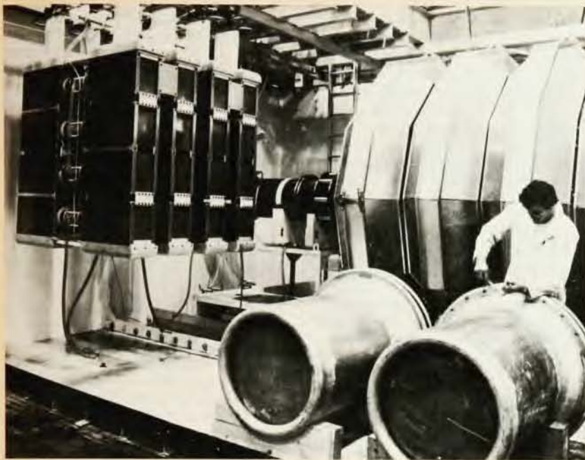
Sandia's radial line accelerator (RADLAC) and Livermore's Advanced Test Accelerator are exploring charged-particle beam technology. In this photo of RADLAC, a generator charges an intermediate storage capacitor (left) to energize the injector. Accelerating voltage is applied synchronously by radial pulse lines (right rear). The accelerating gradient is 5 MeV/meter.
