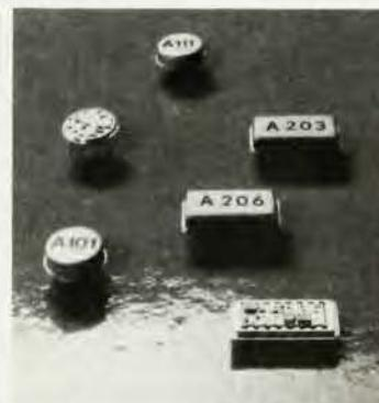
Models A-101 and A-111 are Charge Sensitive Preamplifier-Discriminators developed especially for instrumentation employing photomultiplier tubes, channel electron multipliers (CEM), microchannel plates (MCP), channel electron multiplier arrays (CEMA) and other charge producing detectors in the pulse counting mode.
