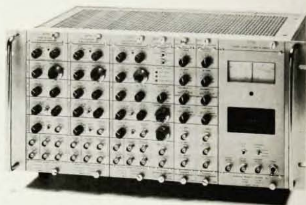
SR280 Mainframe shown with three boxcar modules, a gate scanner module and two analog processors.
