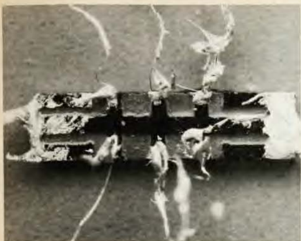
The first observation of the fractionally quantized Hall effect was made by the Bell Labs group with this high-mobility GaAs/AlGaAs heterostructure, 7 mm long and 2 mm wide, at a temperature of about 0.5 K. The dark area contains the two-dimensional electron gas, confined in the interface between GaAs and AlGaAs layers. Current flows in the long direction while Hall voltage is measured across the structure.
