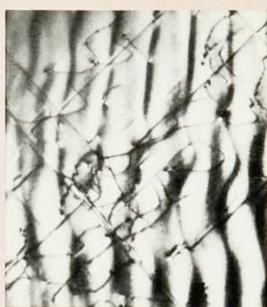
Instability of strained-layer superlattices at high power levels is suggested by the abundance of dislocations seen as fine lines in this micrographic top view of a GaAs/In 0.2 Ga 0.8 As superlattice grown at Varian. Dislocations appeared after it was run as a cw laser photopumped at about 10 3 W/cm 2 . The rippled bands are an artifact.
