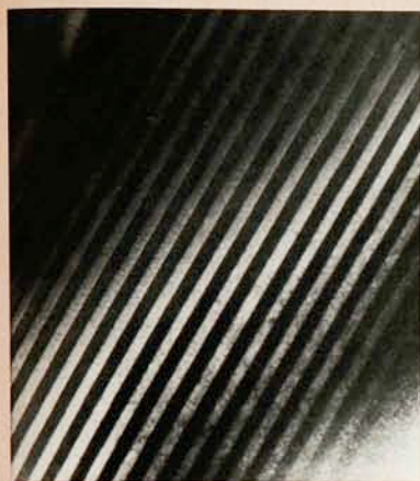
Transmission electron micrograph of a GaP/GaAs 0.28 P 0.72 strained-layer superlattice grown by metal-organic chemical vapor deposition at Sandia by Robert Biefeld and his colleagues. This edge-on view illustrates the uniformity of the 120-Å-thick layers and the lack of dislocations in the superlattice, despite the mismatch of the two materials.
