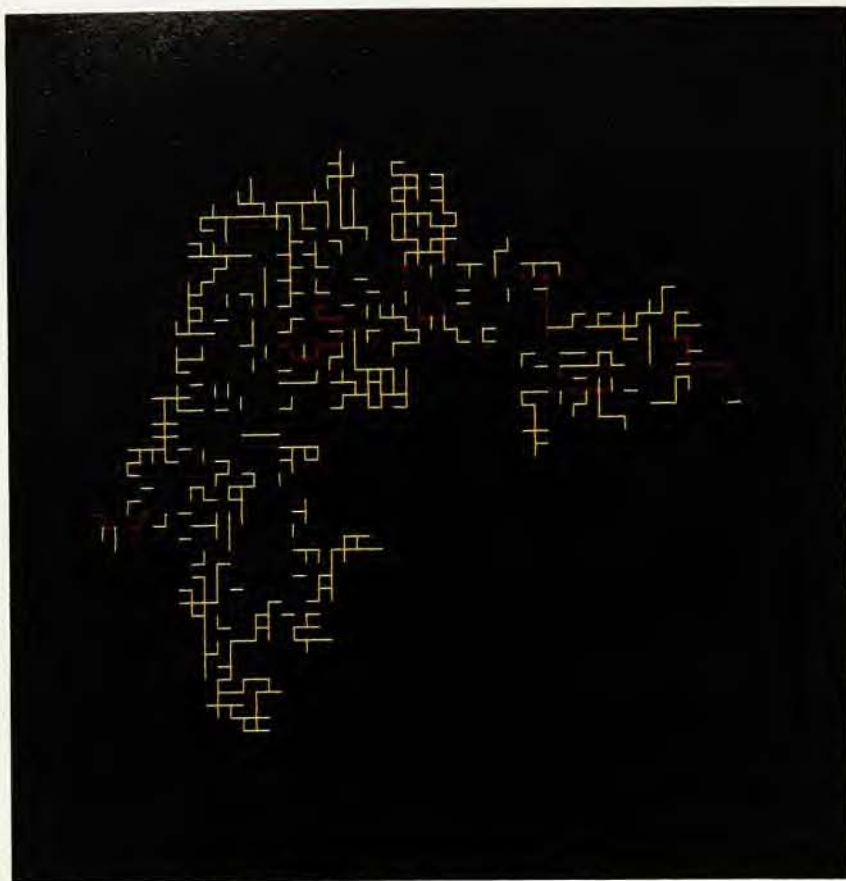
Cluster of connected bonds for the two-dimensional percolation problem, with bond probability 0.45. The bonds were colored by a recursive algorithm made possible by the data structure representing the cluster. If we consider the graph as a resistor network carrying current from the left to the right, the red bonds carry the full current, the blue bonds share the current and the yellow bonds are "dead ends" carrying no current. (After reference 14.) Figure 5
