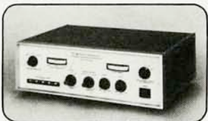
Versatile DTC-500A provides three-term temperature controllability to better than \pm 0.5 millikelvin.
