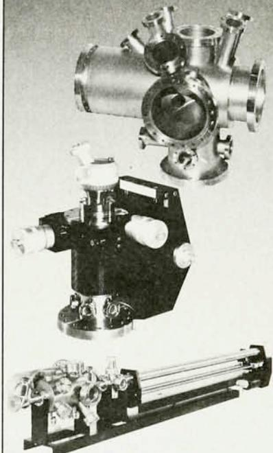
UHV INSTRUMENTS™ manufactures a complete line of precision accessories for the vacuum/surface specialist: precision manipulators, sample insertion and preparation devices, analysis probes, long stroke bellows devices, chambers, shear and tensile fracture devices. These devices can be used to prepare, fracture, transfer, and manipulate samples under vacuum. The accessories are compatible with most commercial analysis systems manufactured by PHI, Varian, HP, VG, Kratos, and others.
