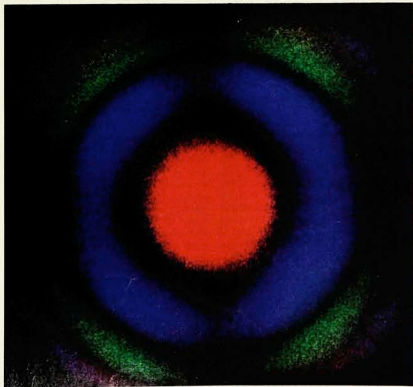
Spontaneous, incoherent synchrotron radiation from the wiggler of the Orsay-Stanford free-electron laser moves from shorter wavelengths (top photo) to longer wavelengths (below) as the magnetic field intensity in the wiggler is increased toward the design value at which laser oscillation will occur. On axis we see the fundamental wavelength, with longer wavelengths emitted at larger off-axis angles. Superposed on this fundamental spectrum is the second-harmonic spectrum, which first becomes visible as the violet ring at larger angle because its central region is in the uv. When the central spot reaches 6500 Å (orange-red), the wavelength at which the mirrors are most reflective, the intensity of the central spot suddenly increases ten-thousand-fold and the surrounding ring pattern vanishes. Coherent laser oscillation has begun.
