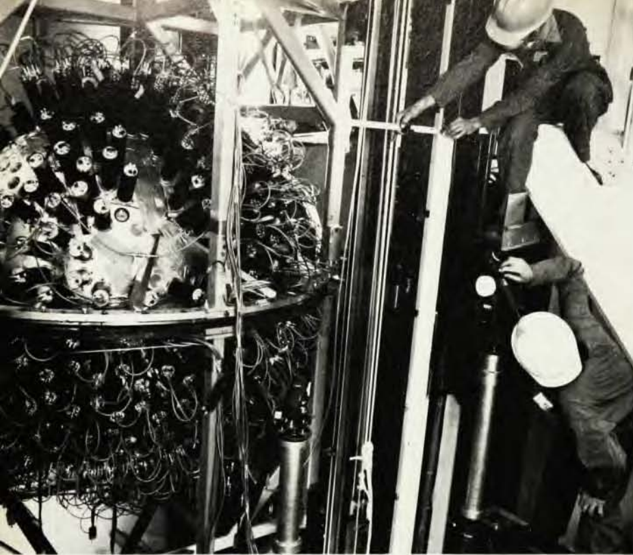
Crystal ball. This particle detector consists of 672 large sodium iodide crystals that are arranged in a sphere 1.32 meters in diameter and surrounded by phototubes. The detector saw use in hadron spectroscopy at the SPEAR storage ring in Stanford. It is now in use at the DORIS II storage ring at DESY in Hamburg. (Courtesy of William W. Ash and Elliott D. Bloom, Stanford Linear Accelerator Center.) Figure 1
