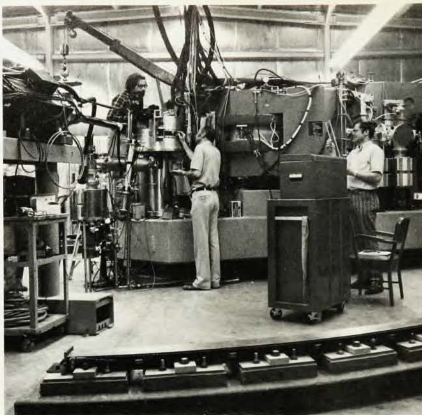
Q3D spectrometer at Los Alamos provides high-precision measurements of the energies of charged particles produced in nuclear reactions. The projectiles come from a tandem Van de Graaff through the tube at left and interact with the target in the chamber being worked on in the center. The spectrometer magnet swings along the track around the target to provide measurements at various angles.
