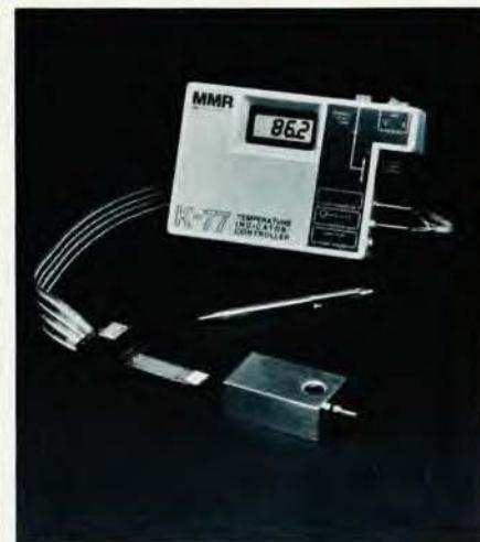
Save lab space, time and scarce research funds by using MMR Technologies' new temperature characterization system to cool small samples and electronic devices from +100°C to -197°C (76K).
