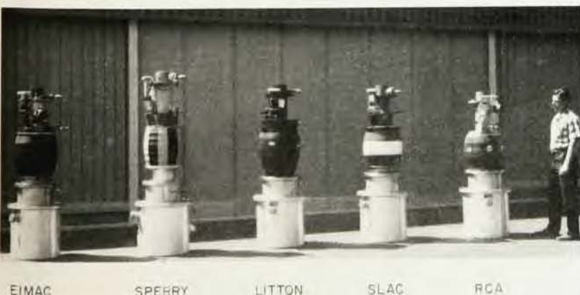
The 250 klystron tubes that supply the rf power for SLAC, have, over the years, been provided by the laboratory's in-house manufacturing facility and four commercial producers.
