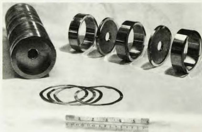
Copper iris disks and rings were brazed together into ten-foot sections in a specially constructed hydrogen furnace to form the SLAC linac accelerating structure. The thin foil rings in the foreground are the brazing material that was placed between the components to be joined.
